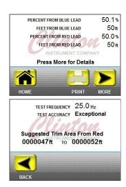
When this setting is ON, the equipment will first locate the distance of the open from the blue probe, and then find its distance from the red probe. A summary screen showing the distance of the fault from each probe will display. The total of the two distances should equal the length of the test cable. By pressing MORE, the operator may view the rated accuracy of the results as well as a suggested cable area to remove. The full report may be printed.
