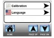
Global settings such as Calibration, Language, and Unit of Measure apply to Opens, Shorts, and Hi-Pot tests. They are found in the several pages of the Settings Menu. To view or modify a setting, press the appropriate button to access the sub screen. Additional screens such as System Information, System Errors, Set System Defaults, and Set Admin Password are also included in the Settings menu.
